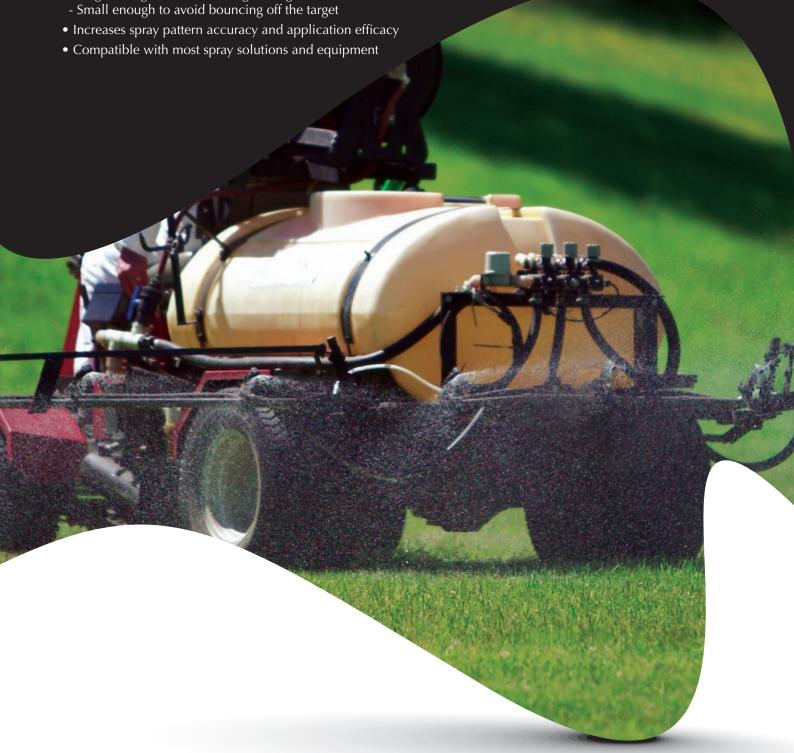
Offside™ improves the accuracy of spray applications by maximizing the percentage of droplets that conform to the ideal size range as they pass through a spray system. Droplets that are larger than the ideal range will tend to bounce off the target surface and deposit the high value pesticide on the soil; those that are smaller than the ideal range may drift onto adjacent sensitive areas with even light winds.
